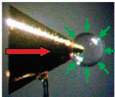
'Fusion target – Green arrows show compression beams - Red arrow the ignition pulse'
